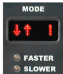
Figure 6.3.1 The MODE window when the radar is in Stationary Mode.
