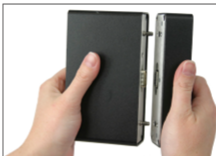
Figure 2.1a Separating the computer/display unit.
