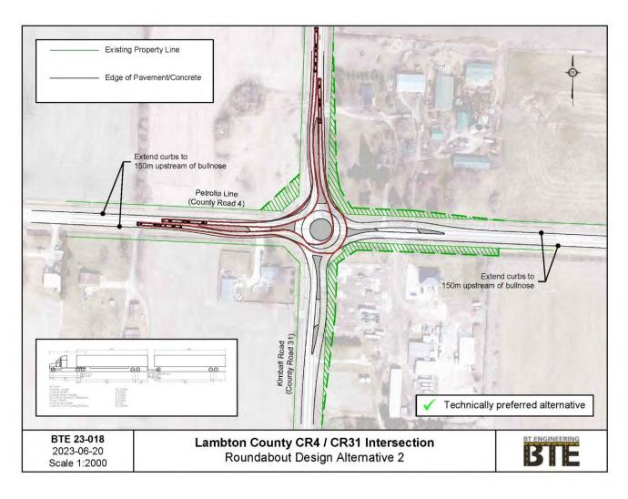
Figure 20: Modified 4-legged Roundabout - Alternative 2
