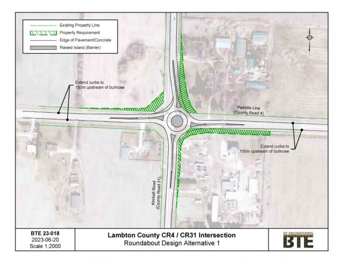
Figure 18: Conventional Roundabout - Alternative 1
