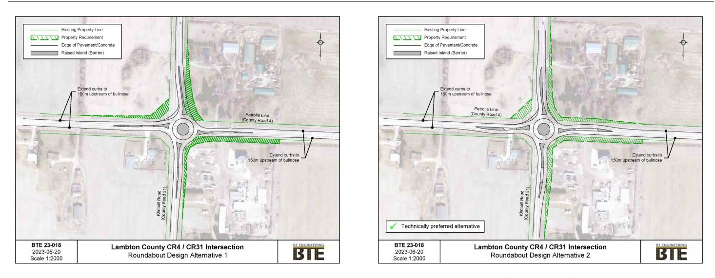
Figure E-3: Roundabout Intersection Alternative 1
