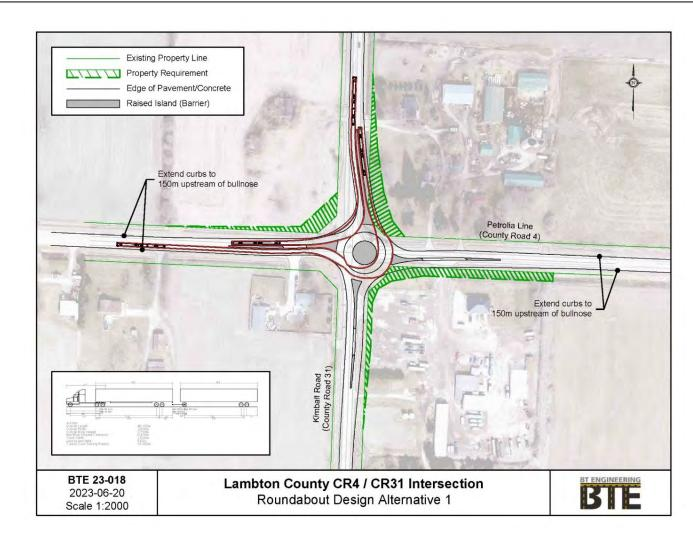
Figure 19: Roundabout Alternative 1 with Large Vehicle Turning Radii
