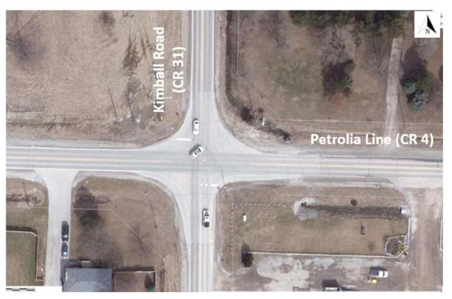
Oversized stop signs with red and white tiger tails for extra visibility, stop ahead signs and Petrolia Line 300m signs are all in place to identify the intersection for northbound and southbound Kimball Road motorists. To provide additional warning for the stop control, rumble strips have been placed on Kimball Road approaching the intersection and a flashing beacon has been placed overhead in the centre of the intersection visible on all approaches, as shown in Photo 1.
