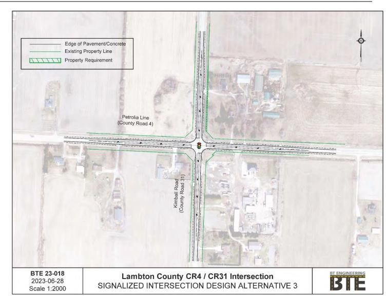
Figure 17: Signalized Intersection
