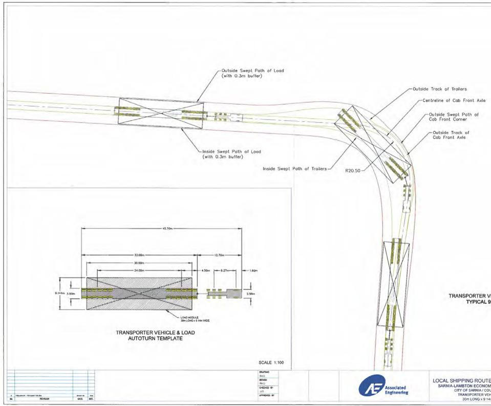
Figure 10: Oversized Load Transporter Vehicle Turning Template
